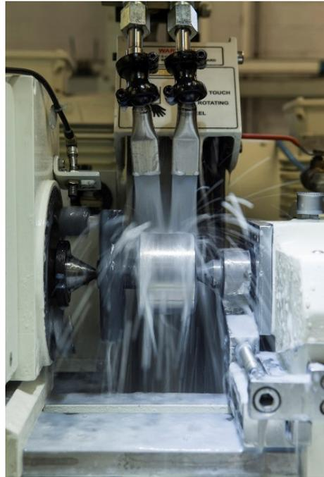
multiple plunges. This series is suitable for grinding gear end or flange end journals of large crankshafts, 6 cylinder or larger. In between the compact, low-cost machines and the heavy duty production grinding machines are a number of machine models which provide solutions to grinding small batches, grinding multiple diameters in one setting, achieving higher material removal rates and higher component accuracy, and others, all of which aim to provide a solution to customer requirements.
