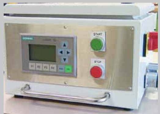
SBA control box automatic for time-regulated cut-in-finishing of individual parts and small series
