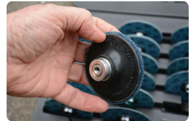
surface conditioning discs and ended up with a surface that was nearly mirror-like. More than I needed for a simple paint job on top, but it was worth a try to see how perfect it could be.
